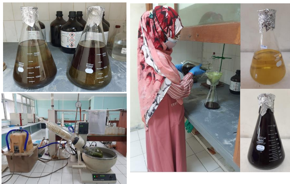
Figure 7. Maceration process of seed powder of Cerbera manghas (left) and Tephrosia vogelii (right) in methanol and ethyl acetate (1:10) (a). The process of filtering the solution and the results of filtering the solutions of C. manghas (top) and T. vogelii (bottom) (b). The process of separating solvents and plant extracts (c).
