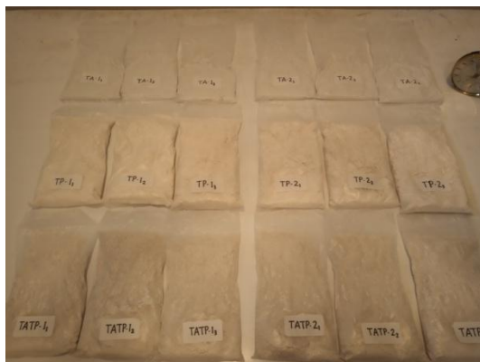
Appendix 8 Storing of yeast powder in various formulations of carrier and additive materials at room temperature ( 28\pm 2 )°C
